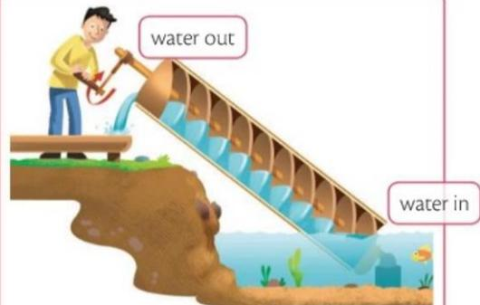
When the mechanism turns, the water moves up the screw and comes out the other end.
